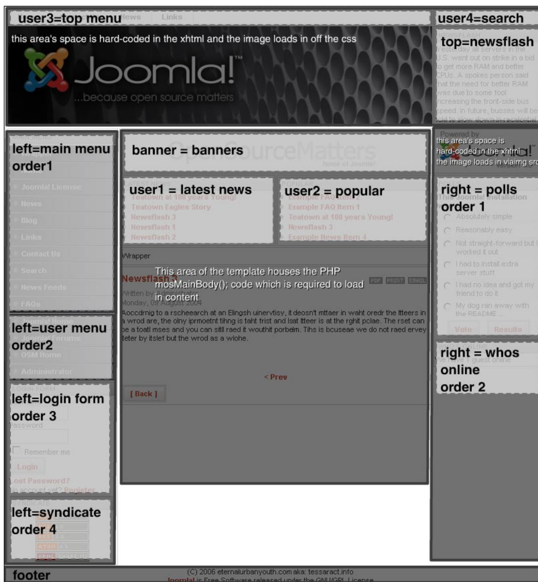
Figure 2.4 Example of modules assigned to Module Positions
