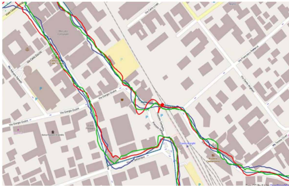
Figure 5. Examples of GNSS trajectories estimated with a Samsung tablet in Como (IT) town
