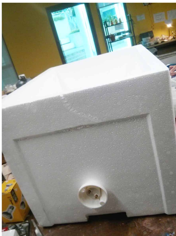
Figure 13. The low-budget incubator uses a simple Styrofoam box as a container
