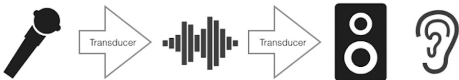
Figure 2.2 Talking and hearing using a process of sensors and transducers.
