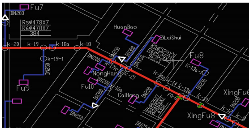
Fig. 2 Distribution of heating substations
